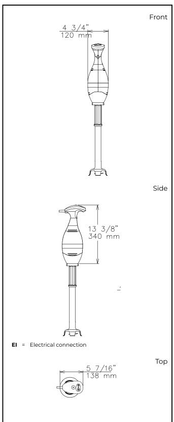
Electric Supply voltage: 602232 (DBP3545U) 110-120 V/1 ph/50/60 Hz **Total Watts:** 0.35 kW Plug type: USA NEMA 5-15P Key Information: External dimensions, Width: 5 7/16" (138 mm) External dimensions, Depth: 4 3/4" (120 mm) External dimensions, Height: 30 1/8" (765 mm) **Shipping width:** 11 7/16" (290 mm) Shipping depth: 27 3/16" (690 mm) **Shipping height:** 7 1/16" (180 mm) **Shipping weight:** 12 lbs (5.3 kg)
